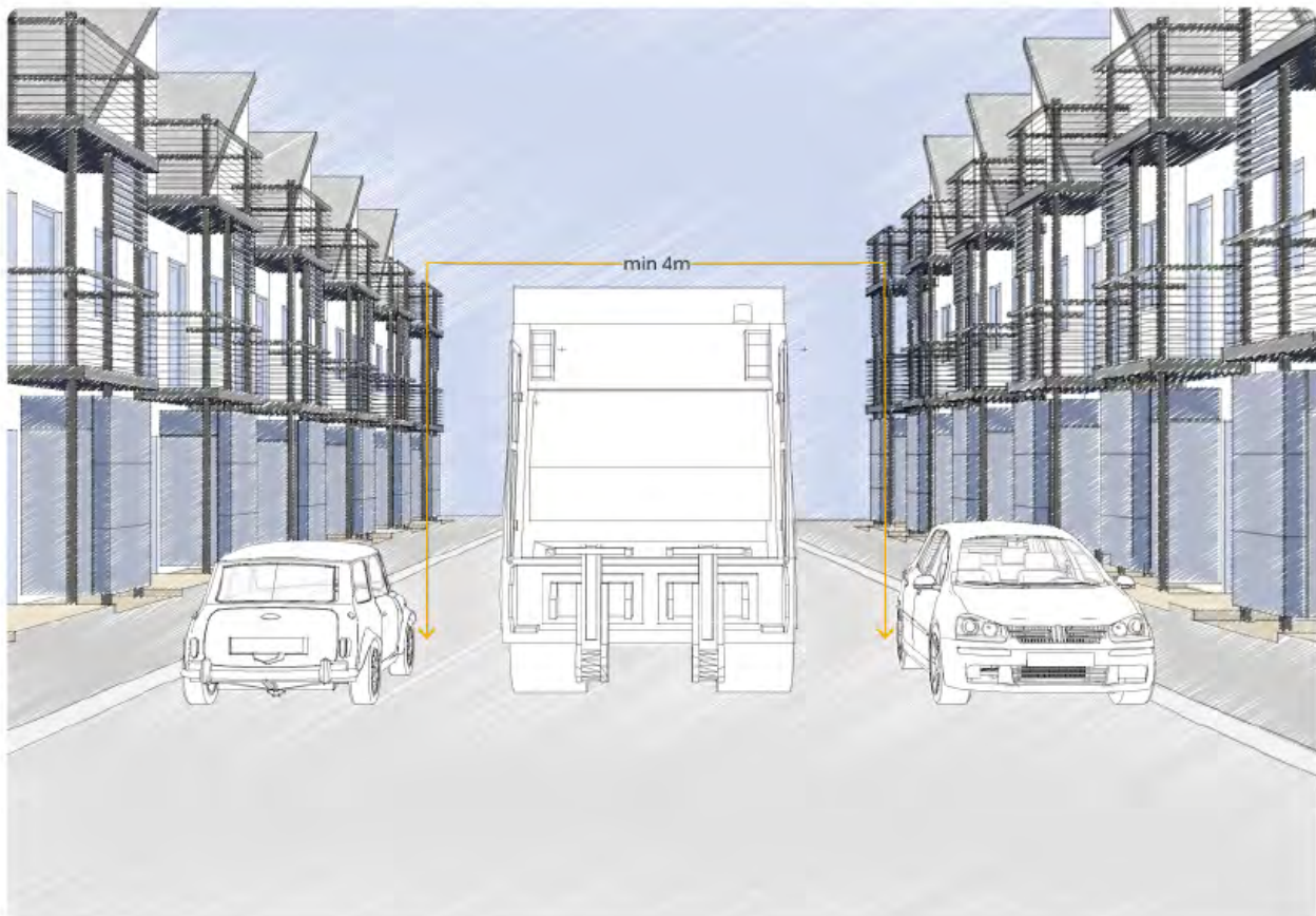
Figure 10 Minimum road width clearance required where on-street parking is provided for on both sides of the road
